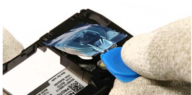
32.) Lever out the Camera Rear Bezel Assy .
