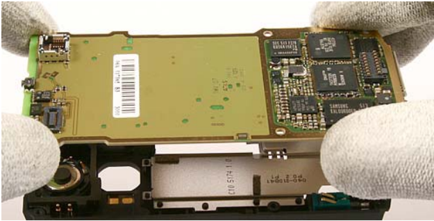
25.) Remove the Engine Module . Place it into the RJ-94 jig immediately.
