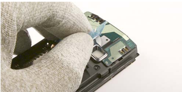
11.) Protect the Camera Rear Bezel Assy with a plastic film before turning the unit.
