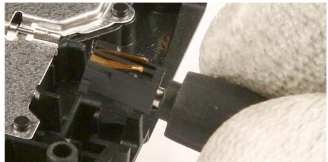
28.) Use the DC plug to remove the DC Jack .
