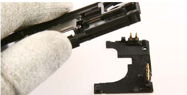
31.) Carefully separate the Antenna Assy .
