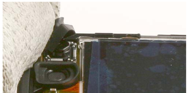
12.) Remove the Camera gasket (N70 only).
