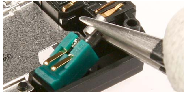
26.) Remove the Vibra Motor with tweezers.
