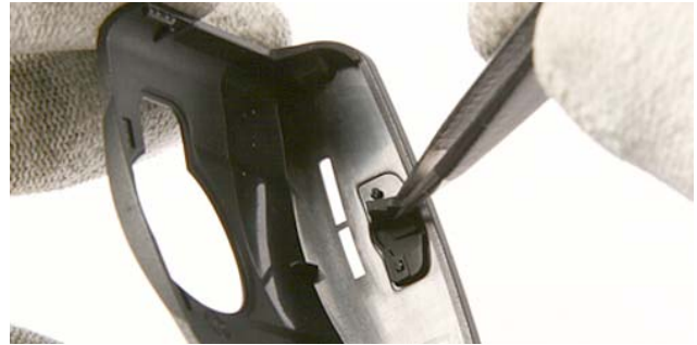
10.) Remove the Power Button with tweezers.
